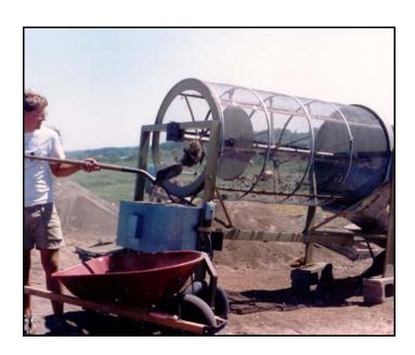
The photograph is of a mechanical screen used at Fort Union, North Dakota by the National Park Service. It was basically a modified grain cleaner, with 1/4 inch mesh on the sides, tiled up so the dirt would sift out and the artifacts and gravels come out into a bucket or wheel barrow on the far end. It worked great in the sandy and gravelly soils, but not so good in clays or hard silts. Artifact recovery was also good, and the artifacts did not appear to be that damaged from the process.
